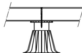
If joists are more than 3m length, we recommend fixing wooden spacers in between to avoid twisting. Therefore, joists are perfectly parallel to each others.
