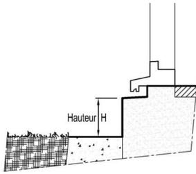
The minimum height H (between the ground level, and the top level of the deck) should be more than 6cm.
