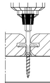
A special bit is provided to allow fastening COBRA® screws between the boards
