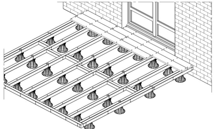
If the ground is not flat, we recommend making a weak mortar to have a stable structure. Before installing the pedestals, spread a **weed control film** of 100gr/m<sup>2</sup> minimum, to prevent growing weeds.
