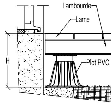
Pedestals should be uniformly positioned under the joists. Spacing will vary depending on the joist thickness.
