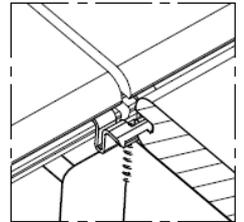
**fiberon®** boards are 100% reversible. Both top and bottom faces are similar. It is possible to turn over the board and use the non-damaged face.
